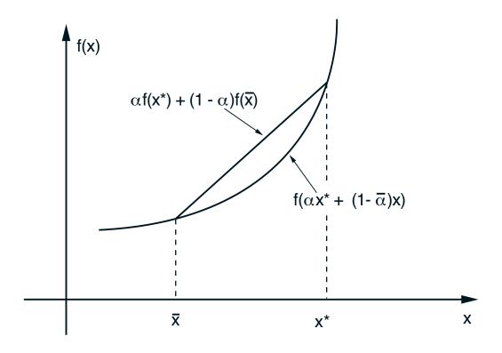
Illustration of why local minima of convex functions are also global. Suppose that f is convex and that  $x^*$  is a local minimum of f. Let  $\overline{x}$  be such that  $f(\overline{x}) < f(x^*)$ . By convexity, for all  $\alpha \in (0,1)$ ,
