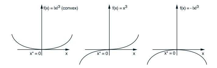
First and second order necessary optimality conditions for functions of one variable.
